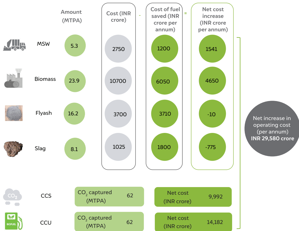
Figure 28 The total OPEX cost is expected to increase with the adoption of alternative fuels
