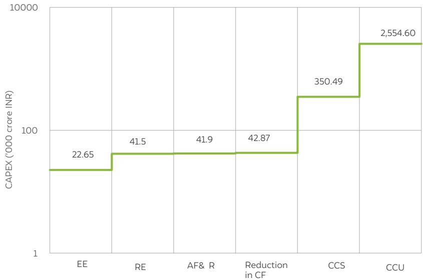
Figure 27 The cost of deploying CCU and CCS requires the highest capital expenditure
